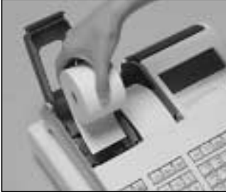
Step 3 Ensuring the paper is being fed from the bottom of the roll, lower the roll into the space behind the printer.
