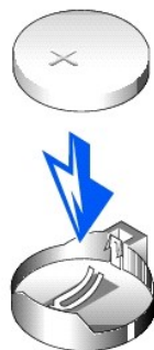
Figure 6-15. Installing the Battery
