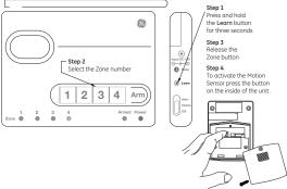
Ensure the Control Center can receive the signal from the intended location of the Sensor before permanently mounting a Sensor.
