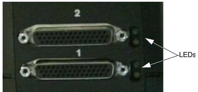
Figure 4-8. V.35/RS-449/RS-530 Network Interface Module (Network Side)
