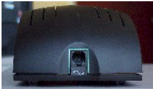
Figure 4-3. Quad BRI Network Interface Module (Peripheral Side)
