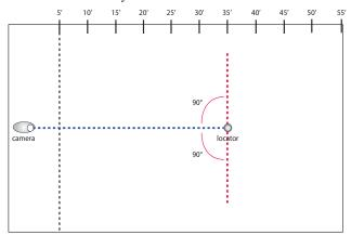
From greater than 35 feet (11 meters) away from the camera, you can face the camera or turn slightly from side-to-side as long as the locator faces no more than 45° away from the center of the camera.
