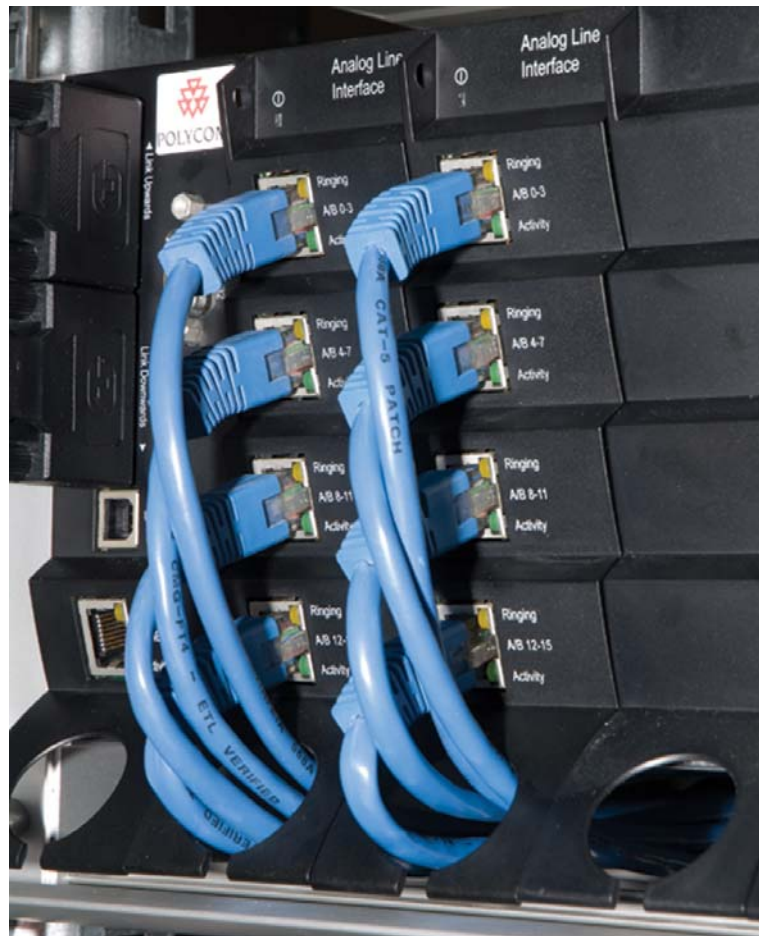
Figure 1-8 Harnessing cables to the back and out
