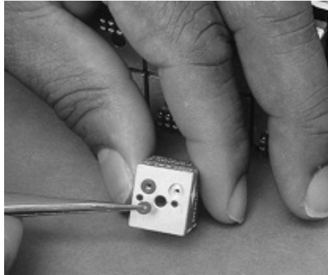
Figure 5.6 DH200 Transducer O-Ring Replacement
