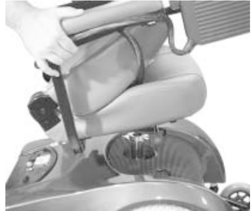
Figure 22. Removing the Seat
