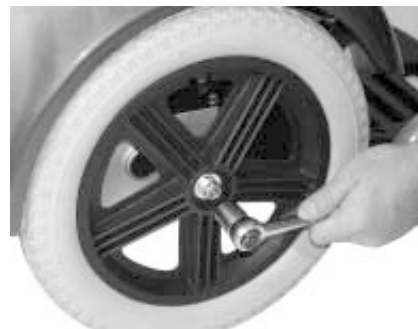
Figure 28. Drive Wheel Nut Removal
