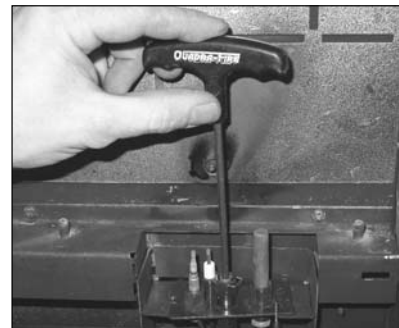
Figure 6.4 Use a 5/32" Allen wrench to remove the pilot injector.
