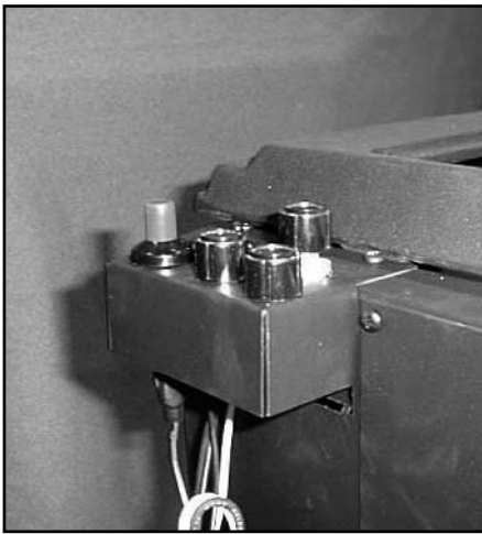
Figure 8.25 Insert the rheostat control into its opening from beneath the control panel. Fit the rheostat nut on top and tighten the nut using an 11/16 in. wrench. Attach the black knob.
