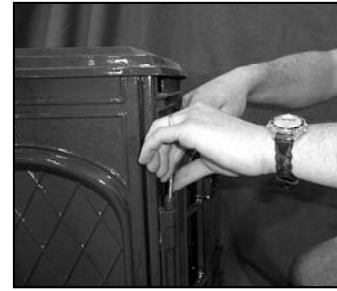
Figure 8.15 Place a washer on the top of the door hinge. Line up the hole in the door hinge and the washer with the hole in the hinge box of the face. Place a gold-plated hinge pin in the hole to secure.
