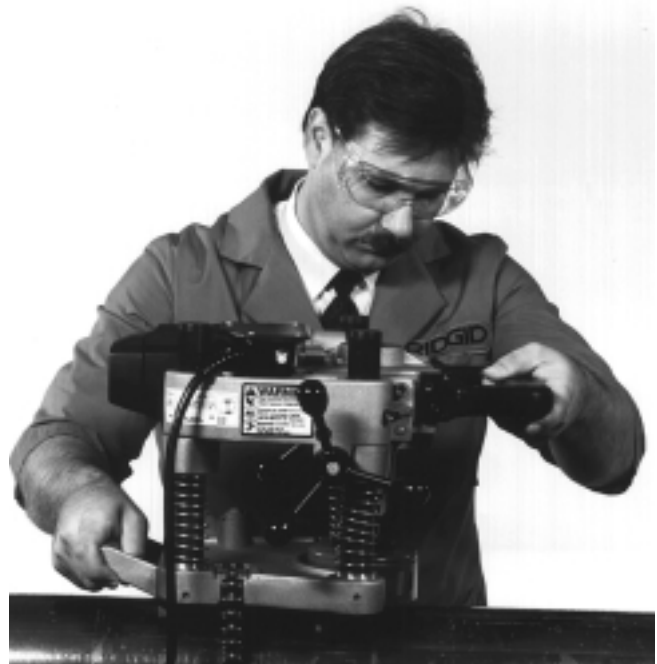
Figure 5 – DO NOT lift HC-450 above your shoulders. May result in loss of balance.
