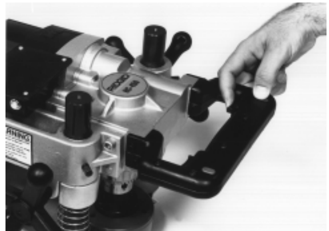
Figure 8 – Model HC-450 Lock Out Switches
