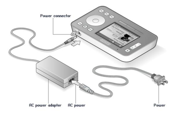
**Caution:** Use only the supplied power adapter to charge the Controller's battery. Using another adapter will damage your Controller and void your product warranty.
