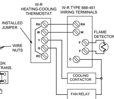
HEATING-COOLING THERMOSTAT WITH SWITCHING SUB-BASE (NOTE: If separate Heating & Cooling Thermostats are used, SPDT Selector switch must be used.)
