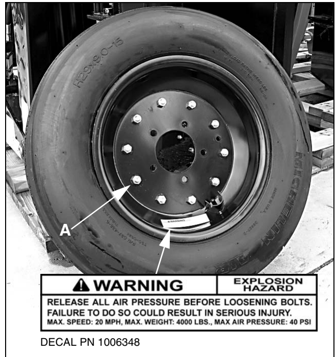
Figure 16. Split Rim Tire Servicing
