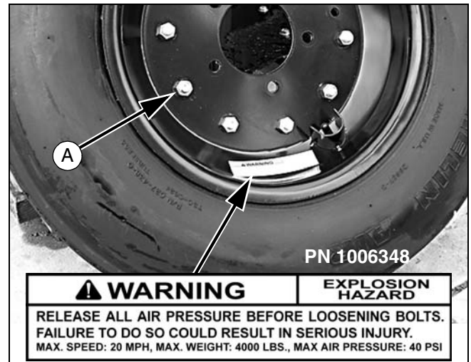
Figure 9. Split Rim Tire Servicing
