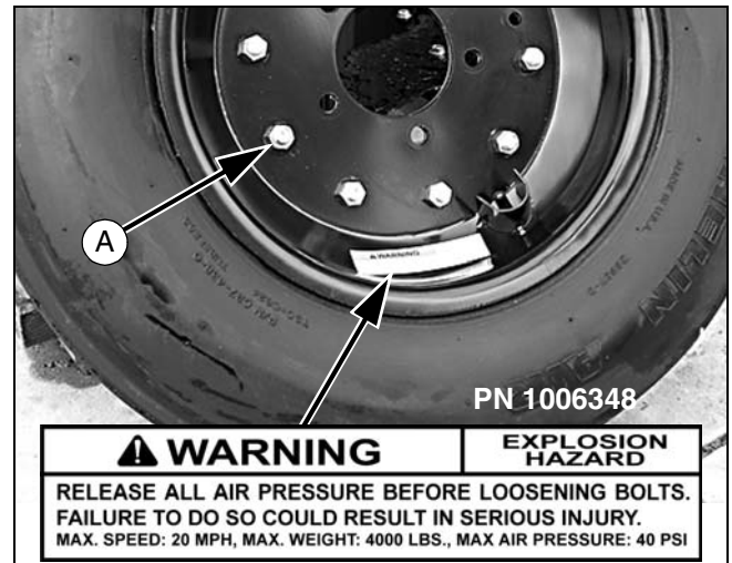
Figure 9. Split Rim Tire Servicing
