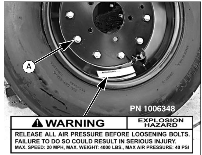
Figure 8. Split Rim Tire Servicing
