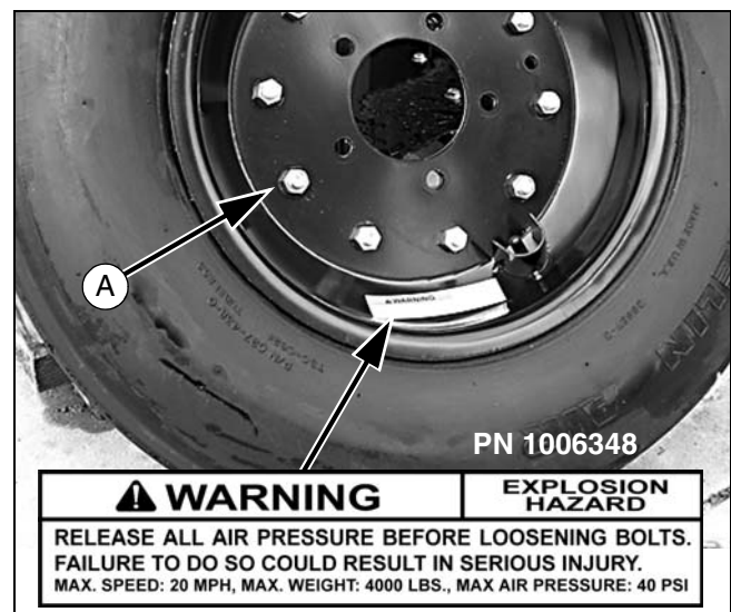
Figure 20. Split Rim Tire Servicing
