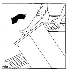
Remove the polystyrene base and take off the bottom panel by unscrewing the central screw.
