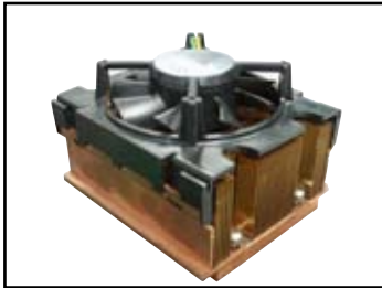
CPU heatsink (top view)
