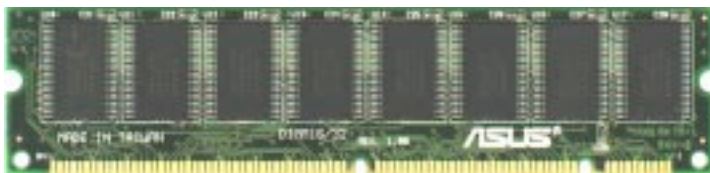
Non-ECC SDRAM DIMM (8 chips)
