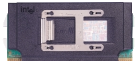
Example of an incorrectly installed retention clip
