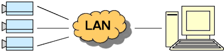
Fig. 4.1 Cameras connected over a local area network to a server PC running DiBos
