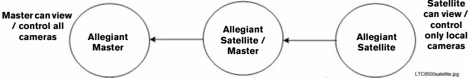
Satellite / Master can view / control local and Satellite's cameras 'Cascaded' Satellite Configuration
