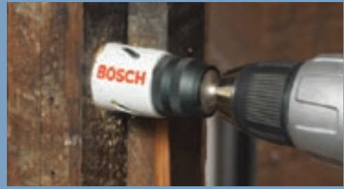
Align saws and re-cut hole
