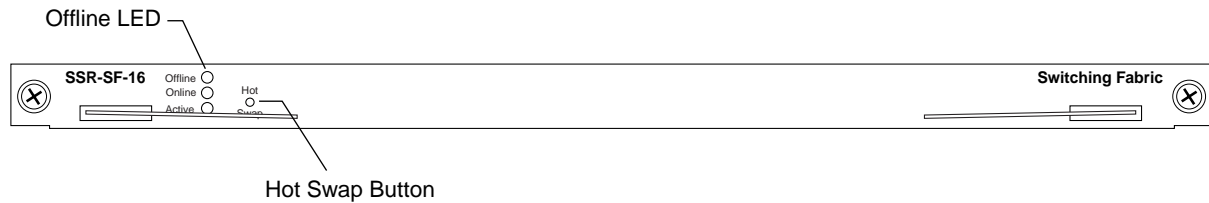
Figure 16. Location of Offline LED and Hot Swap button on a Switching Fabric Module
