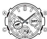
Auto light switch on indicator
