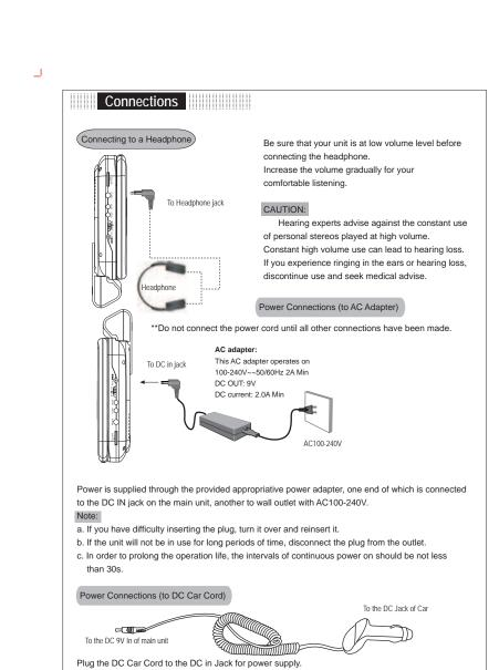
a. Please do not plug it to the battery recharge jack. b. The DC Car Cord is only for in car use.
