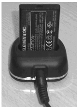
Figure 2-9: Charging the battery
