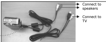
Figure 2-10: Connecting your camera to the TV
