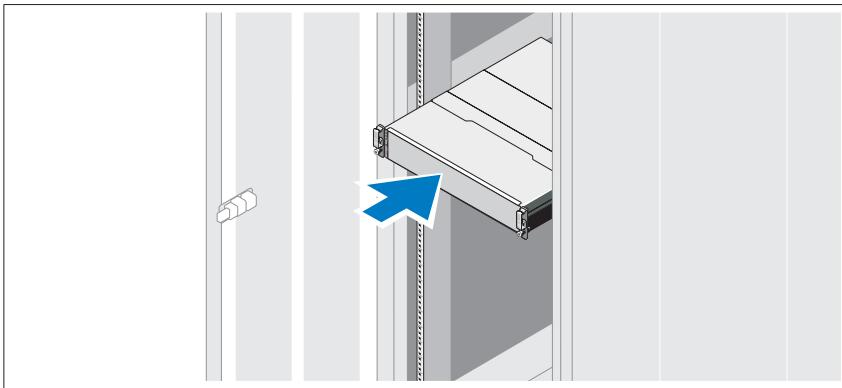
Assemble the rails and install the system in the rack following the safety instructions and the rack installation instructions provided with your system.
