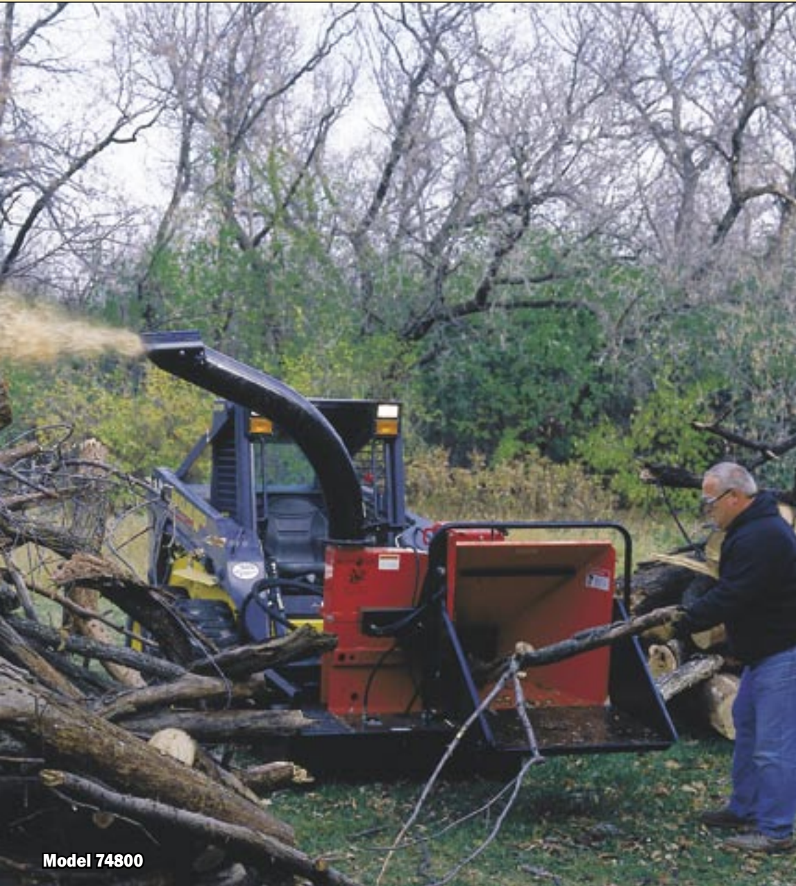
The chipper has two mounts, so it can be set to feed in front or to the curb side.
