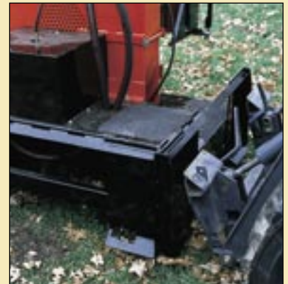
The chipper has two mounts, so it can be set to feed in front or to the curb side.
