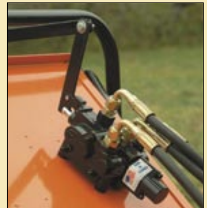
A four-position manual valve easily controls the hydraulic feed roller.
