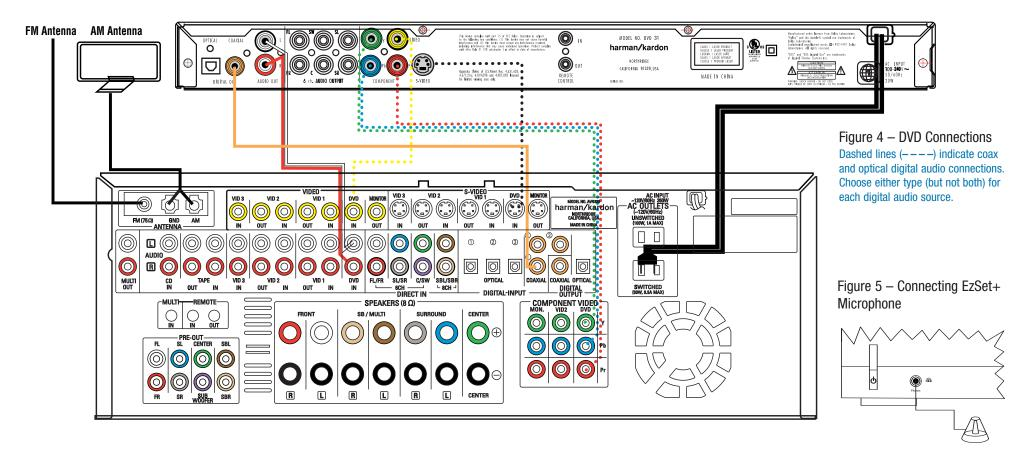
Step 4. Connect AM and FM antennas, as shown above (see page 14). Step 5. Connect the DVD 31 to the AVR 335 as shown above:
