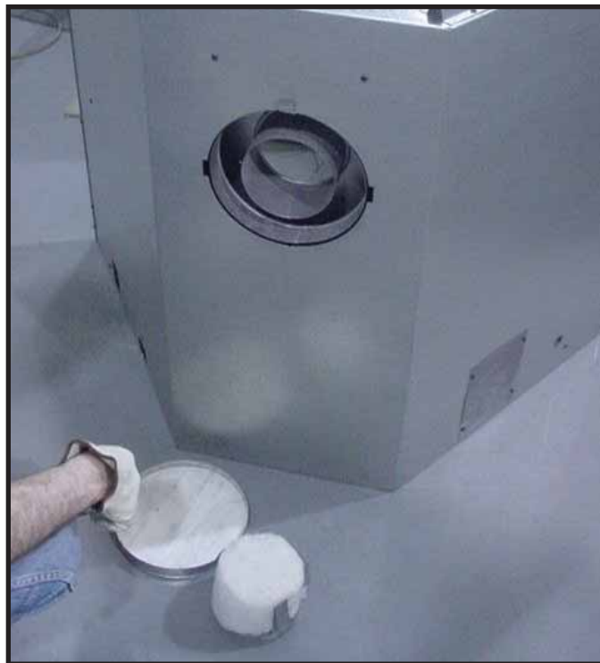
Figure 9.9 Discard the vent cap, remove and discard the insulation basket.
