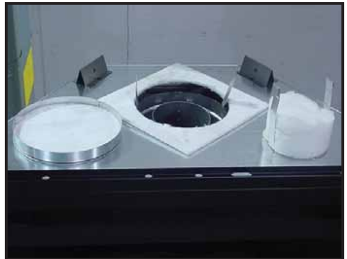
Figure 9.5 Discard the seal cap, remove and discard the insulation basket. Note: Once the vent cap has been removed it cannot be reattached.
