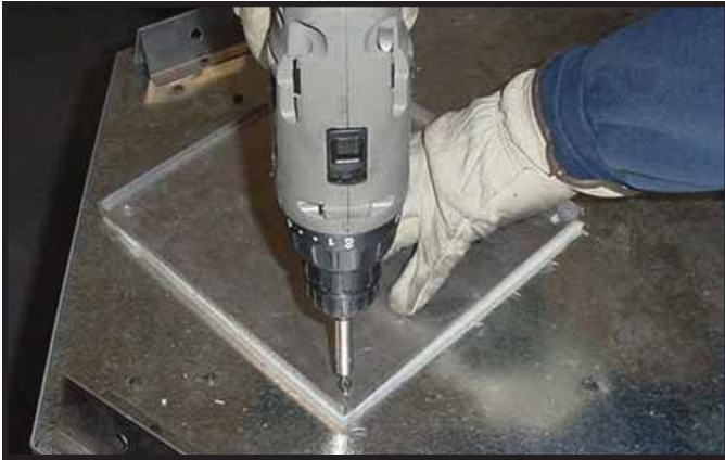
Figure 9.1 Remove the cover plate by removing the four screws holding it to the top of the appliance. Remove and discard the cover plate.
