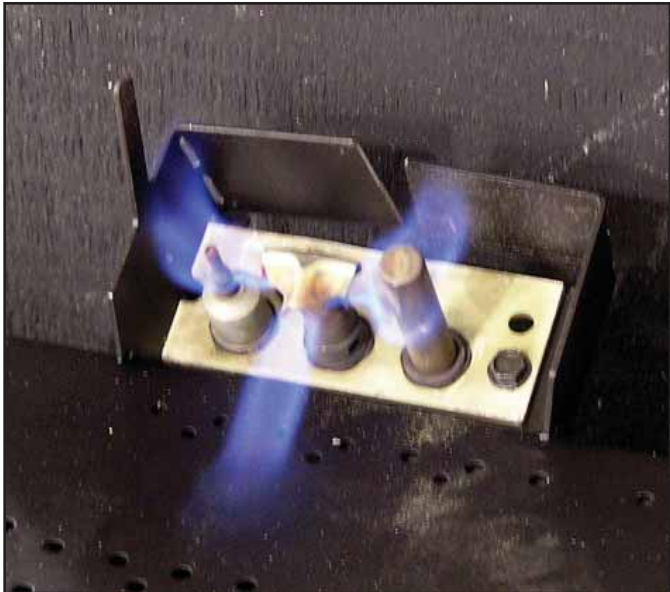
Figure 3.2 Standing Pilot Flame Patterns
