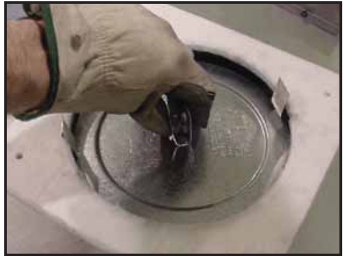
Figure 9.4 Fold the center parts of the retaining band up and use to remove the seal cap.
