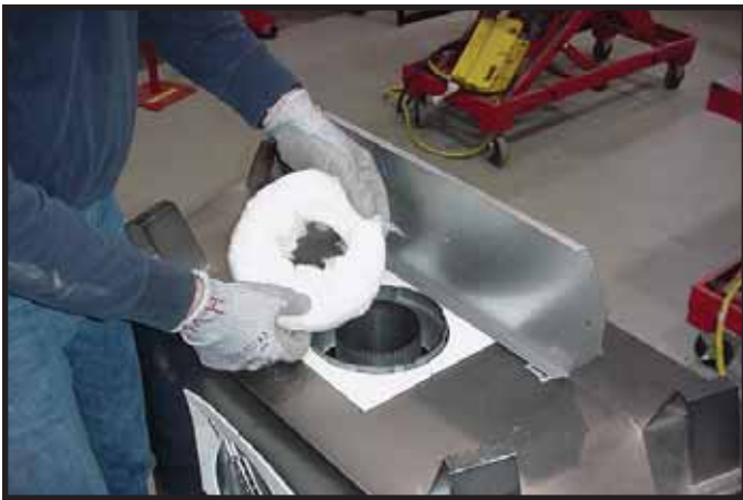
Figure 7.6 Remove the insulation from the outer vent pipe.
