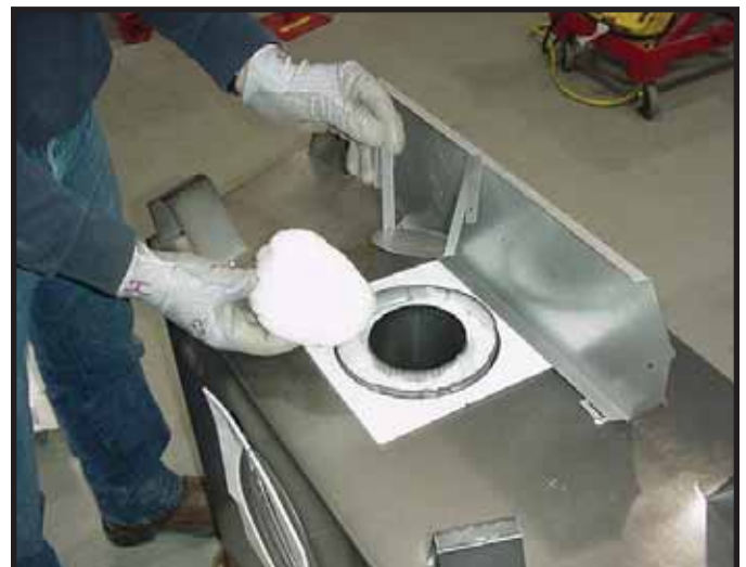
Figure 7.5 Remove the insulation basket and white insulation from the center vent pipe.
