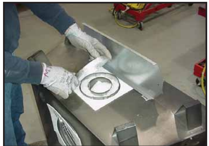
Figure 7.4 Remove the vent cap.
