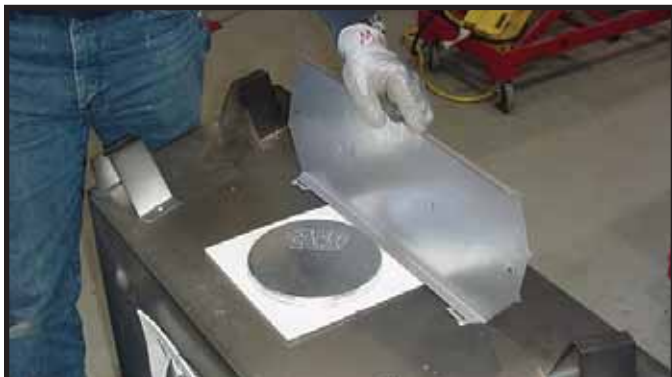
Figure 7.2 Rotate the top heat shield to the vertical position as shown above. The heat shield must remain in the vertical position.
