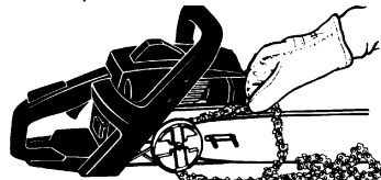
Place chain onto the sprocket
